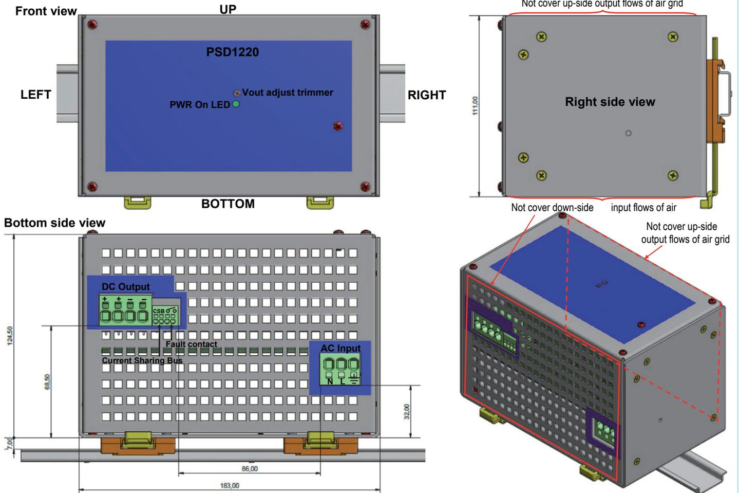
The *PSD1220-098* must only be installed on a DIN-Rail as oriented in the following drawing. All dimensions are in millimeters (mm).
