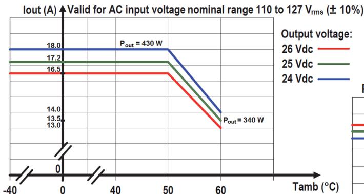
Maximum Output Current & Power vs. Ambient Operating Temperature
