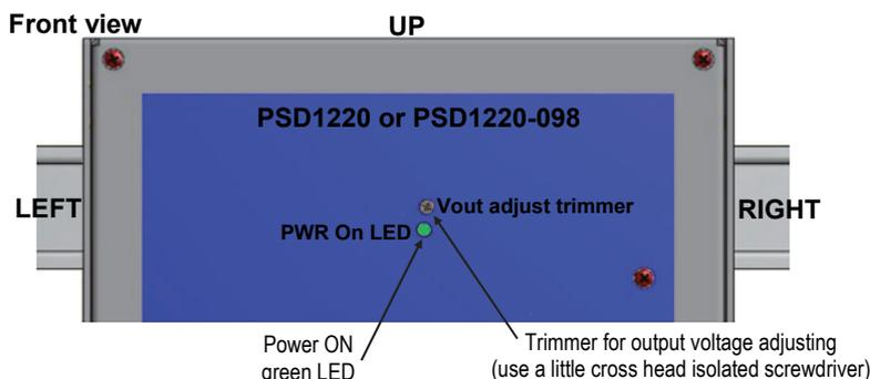
**Pre-Start up:** power the AC mains to turn on PSD1220 or PSD1220-098 unit: Power ON green LED, on front panel, is ON and 24 Vdc (factory setting) output voltage is present on DC output terminal block.
