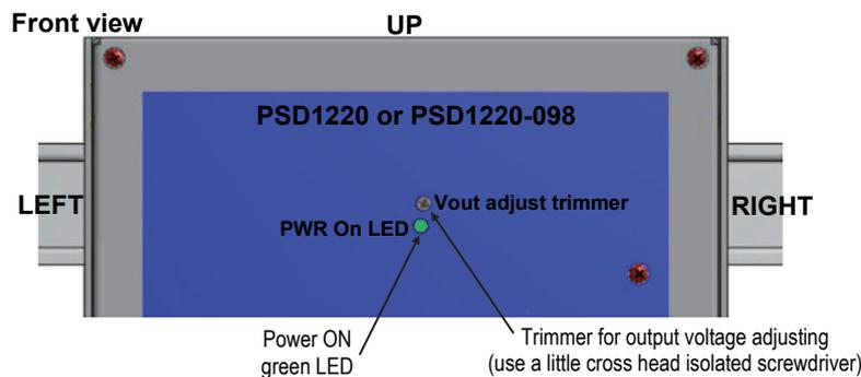
**Start up:** power the AC line to turn on PSD1220 or PSD1220-098 unit: Power ON green LED, on front panel, is ON and 24 Vdc (factory setting) output voltage is present on DC output terminal block.
