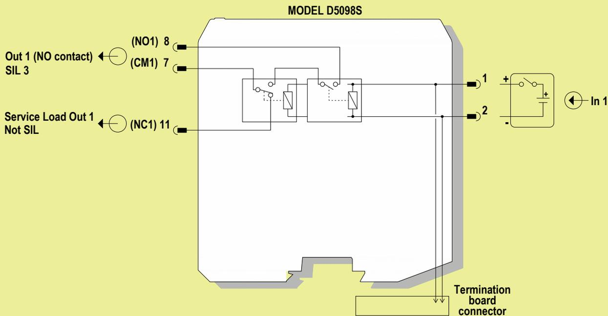
Relay contacts shown in de-energized position. Terminals 7-8 are open; terminals 7-11 are closed.
