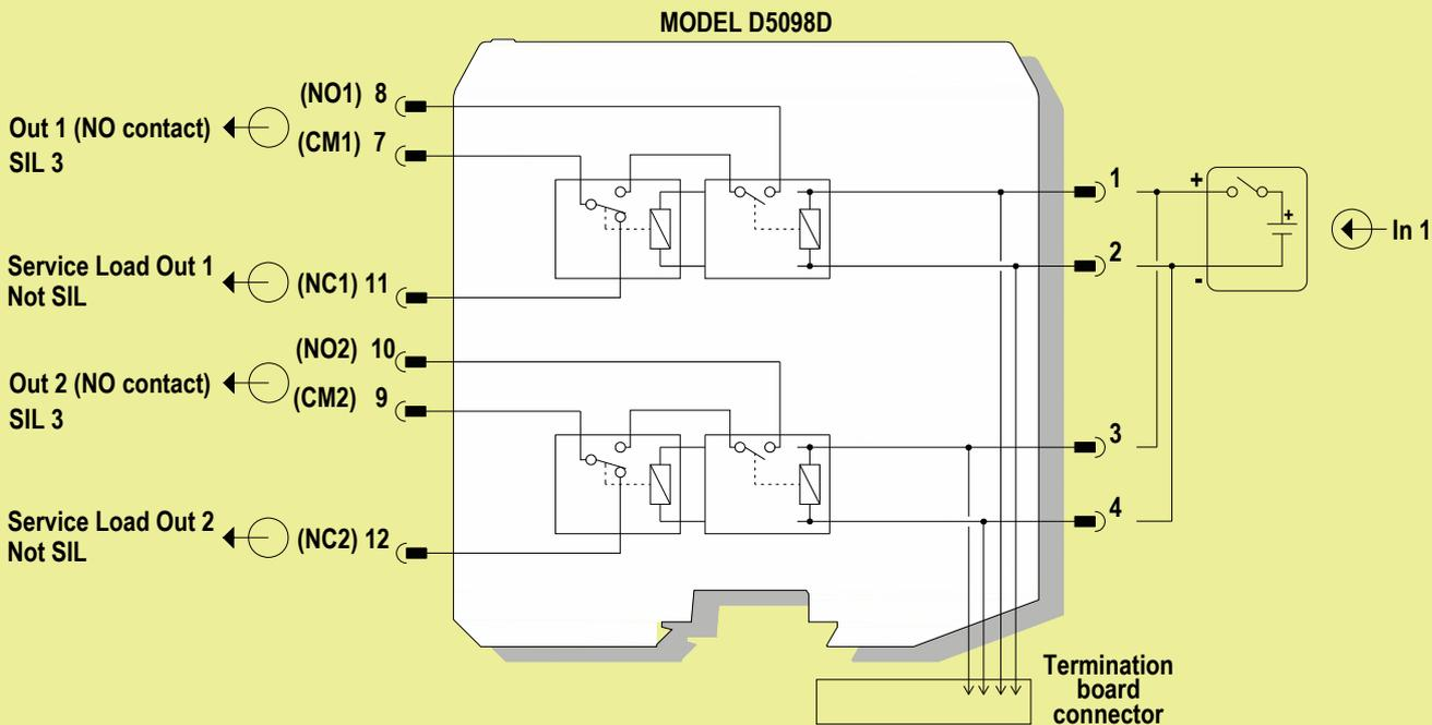
Relay contacts shown in de-energized position. Terminals 7-8 and 9-10 are open; terminals 7-11 and 9-12 are closed.
