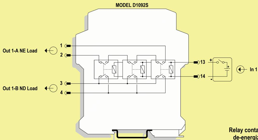
**To prevent relay contacts from damaging, connect an external protection (fuse or similar),
