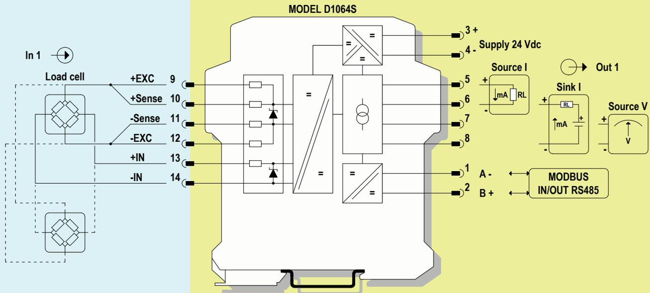
Up to 4 load cells 350  $\Omega$  in parallel
