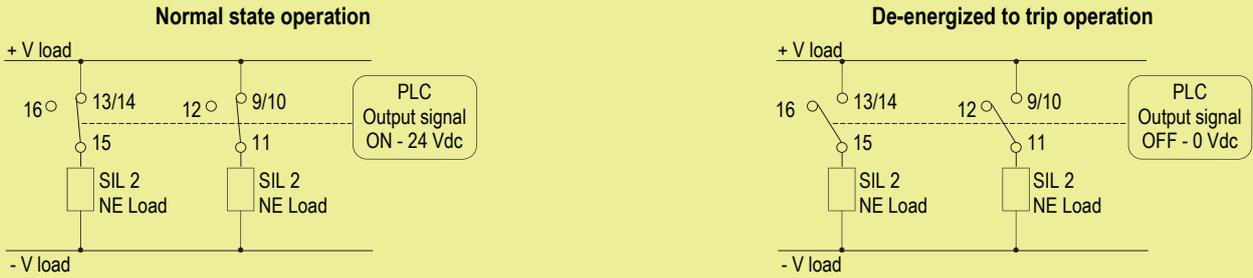
SIL 2 Normally Energized Relay Condition for ND Load
