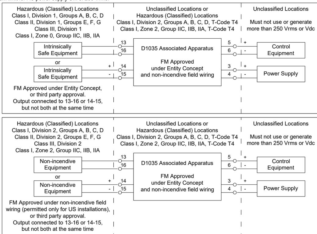
Non-incendive field wiring is not recognized by the Canadian Electrical Code, installation is permitted in the US only.
