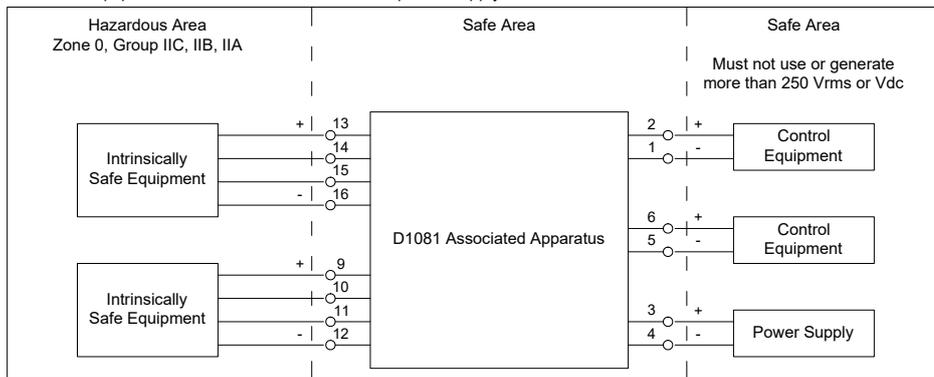
Not to be connected to control equipment that uses or generates more than 250 Vrms with respect to earth ground.
