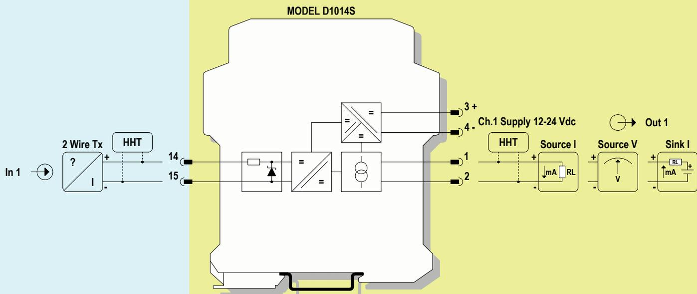
Application for D1014S or D1014D, with passive input (2 wires Tx)
