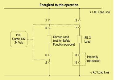
Contacts 1-5 and 2-6: closing of this contact can be used to monitor contacts 3 - 7. Service load (not for Safety Function purpose) is energized.
