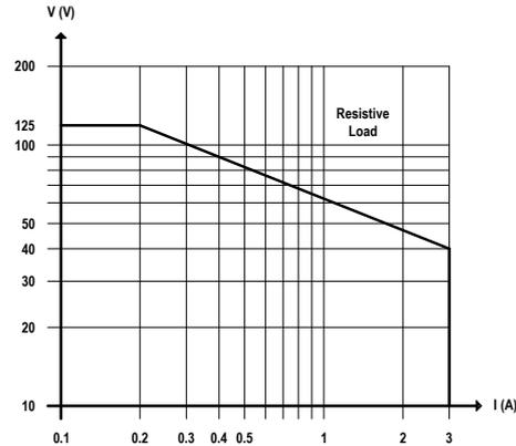
**Mechanical / Electrical life:** 50 \* 10<sup>6</sup> / 1 \* 10<sup>5</sup> operation, typical.
