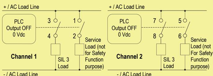
**Contacts 1-2 and 5-6:** in normal operation the relay is de-energized, contacts are open, Service Load loads (not for Safety Function purpose) are de-energized.
