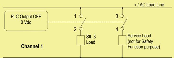
**Contacts 1-2:** the SIL 3 Safety Function is met when the relay is de-energized, contact is open, SIL 3 load is de-energized.
