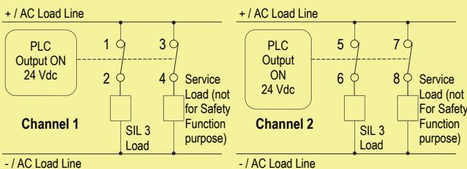
**Contacts 1-2 and 5-6:** in normal operation the relay is energized, contacts are closed, SIL 3 loads are energized.
