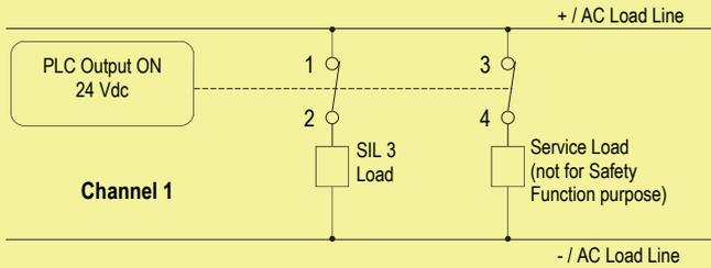
**Contacts 1-2:** in normal operation the relay is energized, contact is closed, SIL 3 load is energized.
