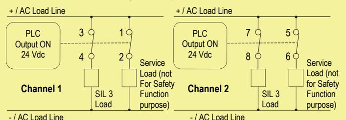
**Contacts 1-2 and 5-6:** closing of these contacts can be used to monitor contacts 3 - 4 and 7-8. Service loads (not for Safety Function purpose) are energized
