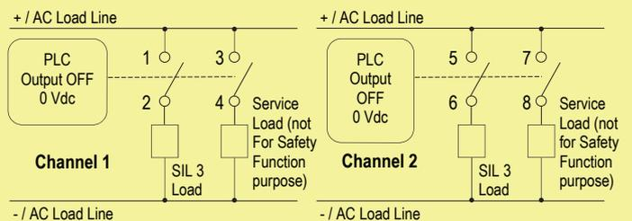
**Contacts 1-2 and 5-6:** the SIL 3 Safety Function is met when the relay is de-energized, contacts are open, SIL 3 loads are de-energized.
