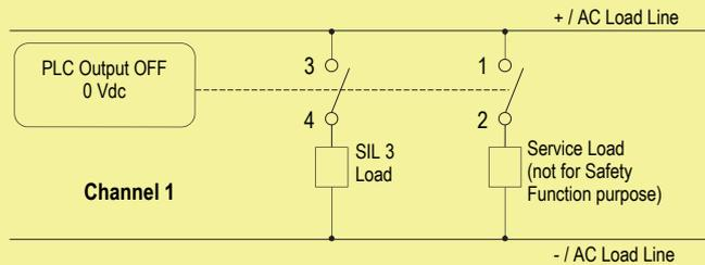
**Contacts 1-2:** in normal operation the relay is de-energized, contact is open, Service Load load (not for Safety Function purpose) is de-energized.
