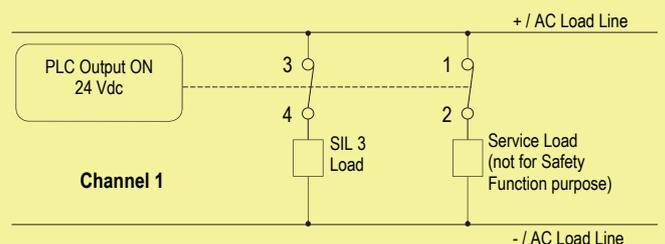
**Contacts 1-2:** closing of this contact can be used to monitor contacts 3 - 4. Service load (not for Safety Function purpose) is energized.
