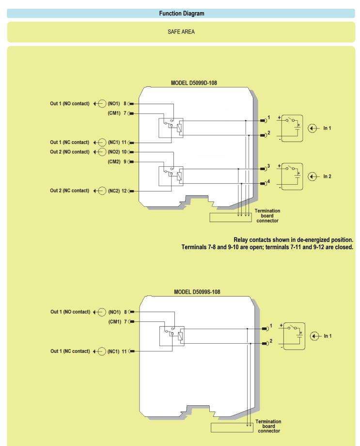
Relay contacts shown in de-energized position. Terminals 7-8 are open; terminals 7-11 are closed.
