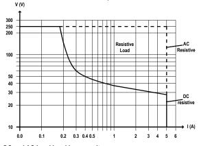
DC and AC Load breaking capacity: Mechanical / Electrical life: 5 \* 10<sup>6</sup> / 3 \* 10<sup>4</sup> operation, typical. Operate / Release time: 6 ms / 12 ms typical, including contact bounce time.
