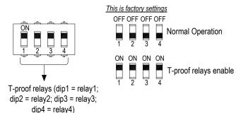
WARNING: after T-proof test, dip-switch 1-2-3-4 must be set to "OFF" position for normal operation.
