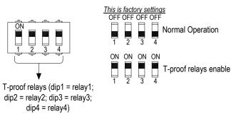
WARNING: after T-proof test, dip-switch 1-2-3-4 <u>must be</u> set to "OFF" position for normal operation.
