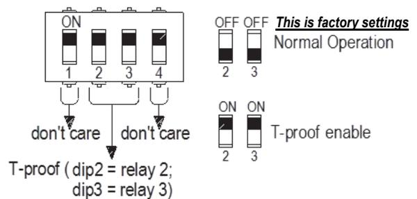
**WARNING:** after T-proof test, dip-switch 2-3 **must be set** to "OFF" position for normal operation.
