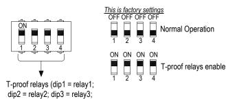
WARNING: after T-proof test, dip-switch 1-2-3-4 <u>must be</u> set to "OFF" position for normal operation.
