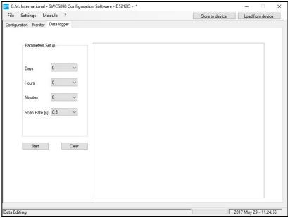
Figure 67: Data Logger screen.
