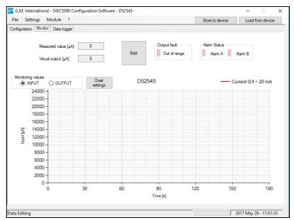
Figure 61: D5254S / D6254S Monitor screen.
