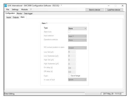
Figure 65: D5212Q / D6212Q Alarm configuration screen.
