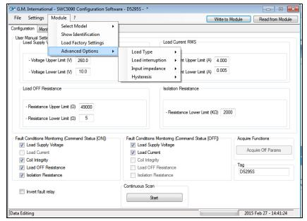
Figure 50: D5294S, D5295S Advanced configuration options.
