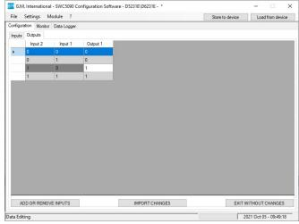
Figure 30: D5231E / D6231E custom function configuration.
