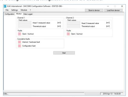
Figure 23: D5072D-096 Monitor screen.
