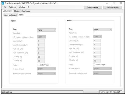
Figure 60: D5254S / D6254S Alarm configuration screen.
