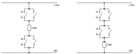
Figure 44: Bipolar (on the left) and unipolar (on the right) load interruption.
