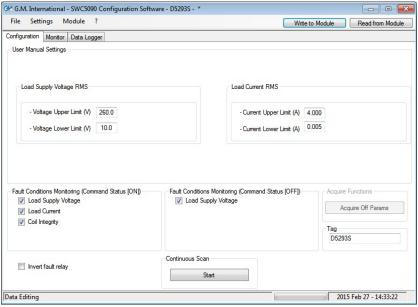
Figure 42: D5293S Configuration screen.
