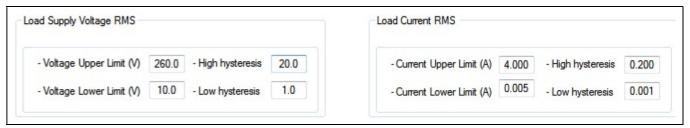
Figure 45: D5293S with Hysteresis enabled.
