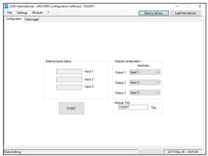
Figure 33: D5240T configuration screen.
