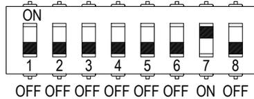
3) short circuit fault detection:
