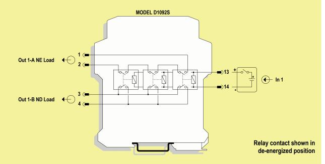
To prevent relay contacts from damaging, connect an external protection (fuse or similar), chosen according to the relay breaking capacity diagram.
