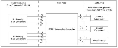
Not to be connected to control equipment that uses or generates more than 250 Vrms or Vdc with respect to earth ground.
