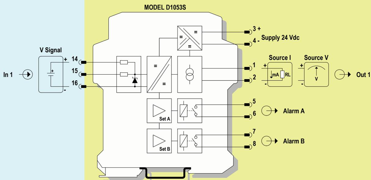
For SIL applications, alarm contacts must be used in series with equal configuration. Relay contact shown in de-energized position
