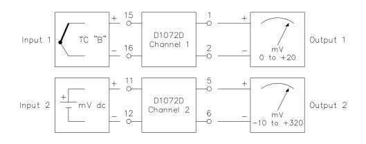
Note: Power supply connection not shown on the diagram
