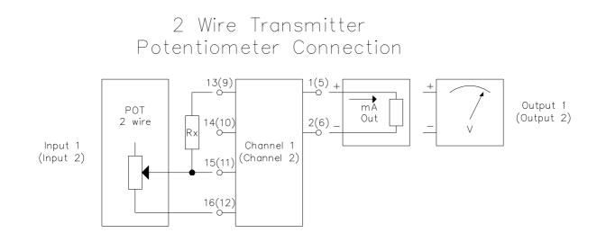
Rx Value: must be equal to the end to end resistance of the potentiometer to obtain 50% full scale value.
