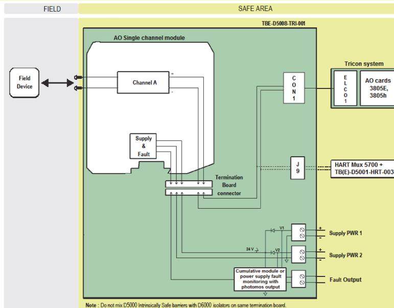
The diagram shows a single channel module on TBE. On a single TBE-D5008-TRI-001 Termination Board can be installed up to 8 single ch. modules for a maximum of 8 channels.
