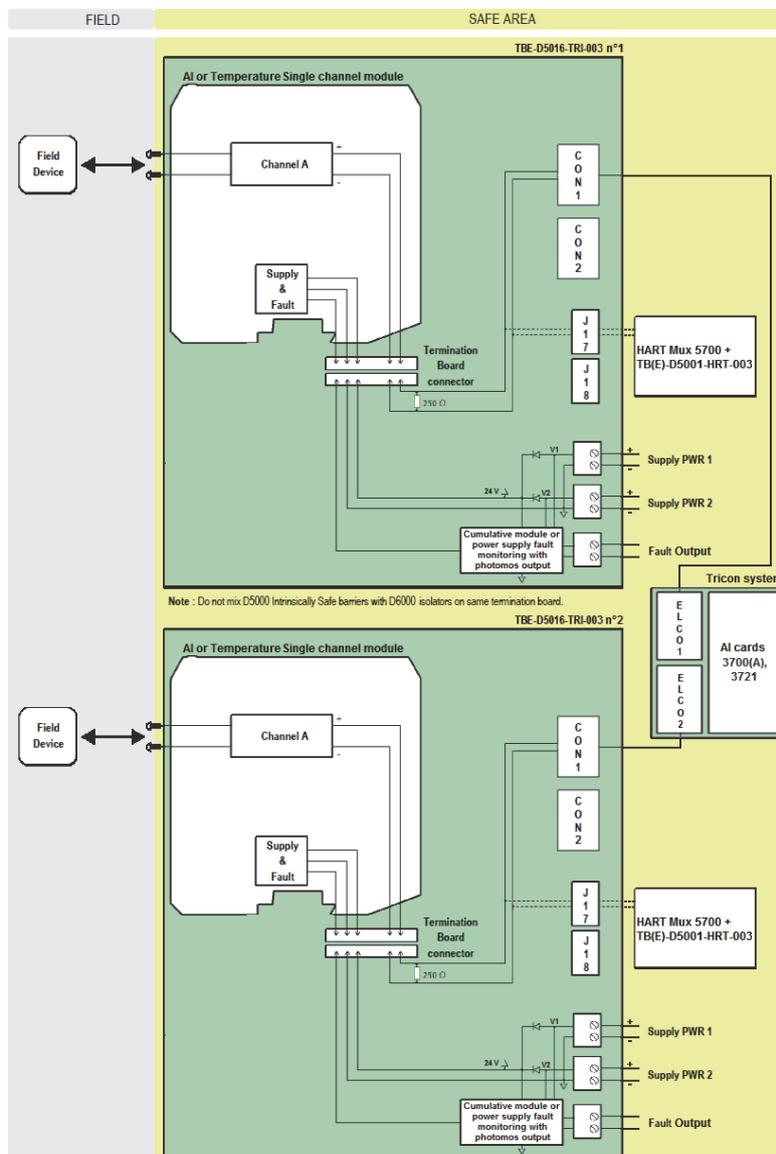
The diagram shows a single channel module on each TBE. On two TBE-D5016-TRI-003 Termination Boards can be installed up to 16+16 single channel modules for a maximum of 32 channels.
