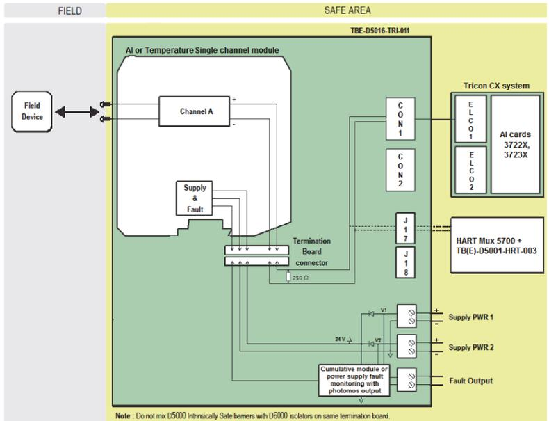
The diagram shows a single channel module on TBE. On a single TBE-D5016-TRI-011 Termination Board can be installed up to 16 single ch. modules for a maximum of 16 channels.
