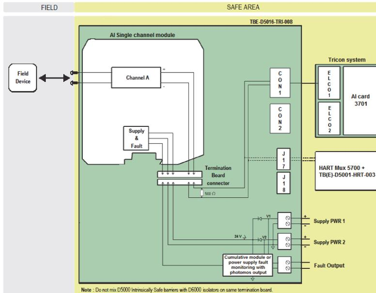
The diagram shows a single channel module on TBE. On a single TBE-D5016-TRI-008 Termination Board can be installed up to 16 single ch. modules for a maximum of 16 channels.
