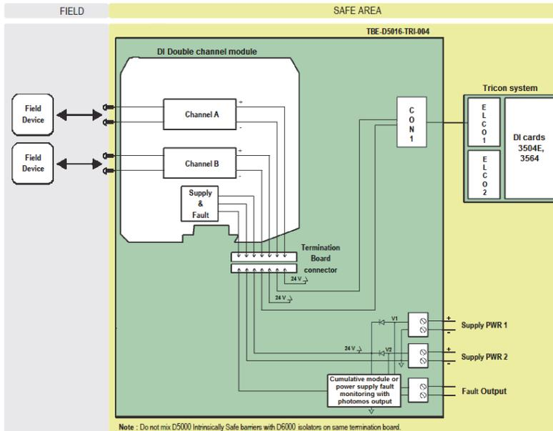
The diagram shows a double channel module on TBE. On a single TBE-D5016-TRI-004 Termination Board can be installed up to 16 double ch. modules for a maximum of 32 channels.
