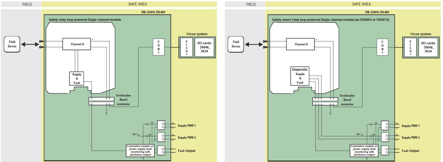
Each diagram shows a single channel module on TBE.
