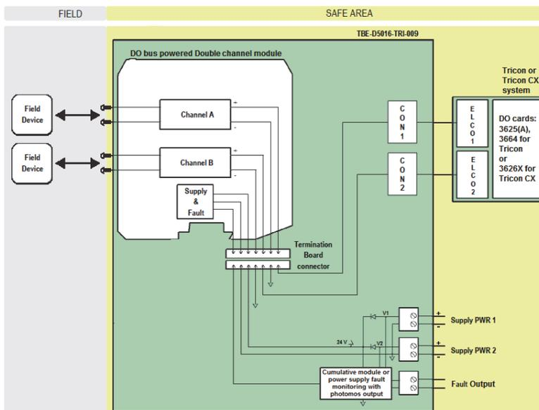
The diagram shows a double channel module on TBE.
