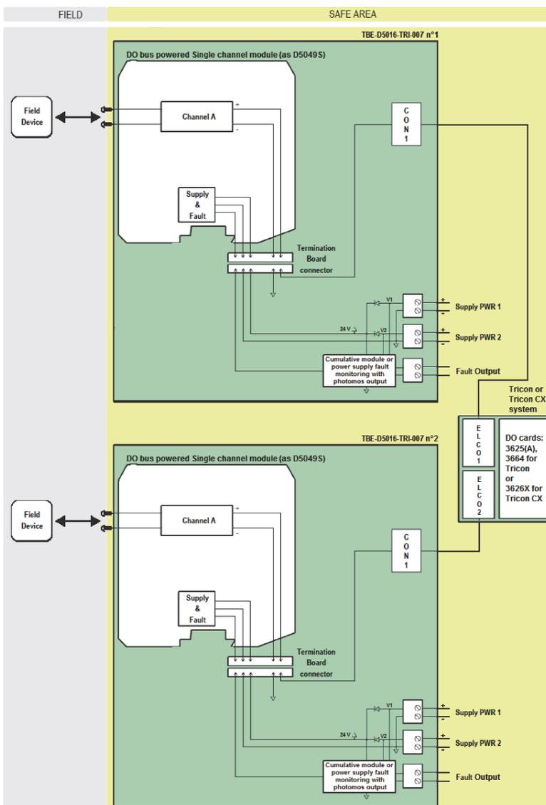
The diagram shows a single channel module on each TBE.
