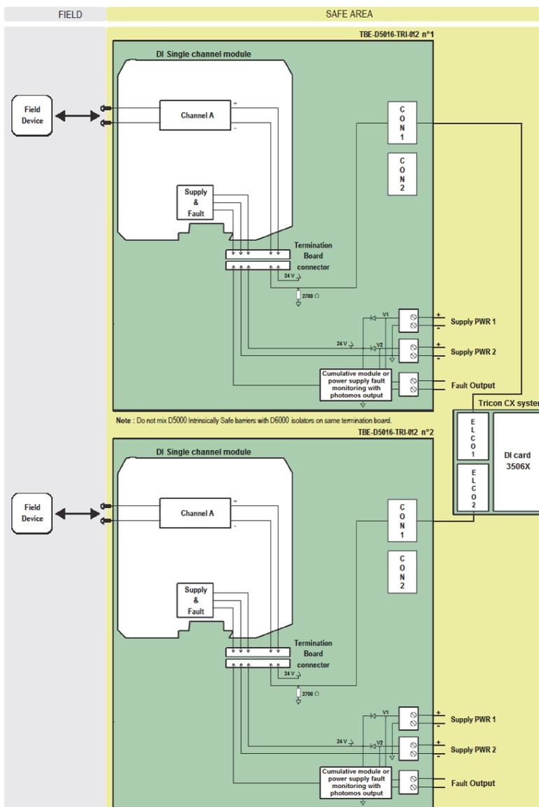
The diagram shows a single channel module on each TBE. On two TBE-D5016-TRI-012 Termination Boards can be installed up to 16+16 single channel modules for a maximum of 32 channels.
