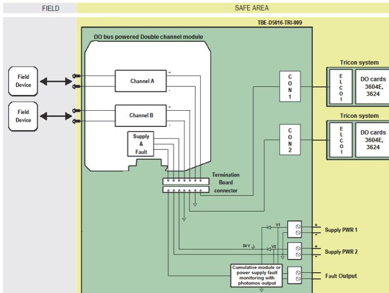
The diagram shows a double channel module on TBE.
