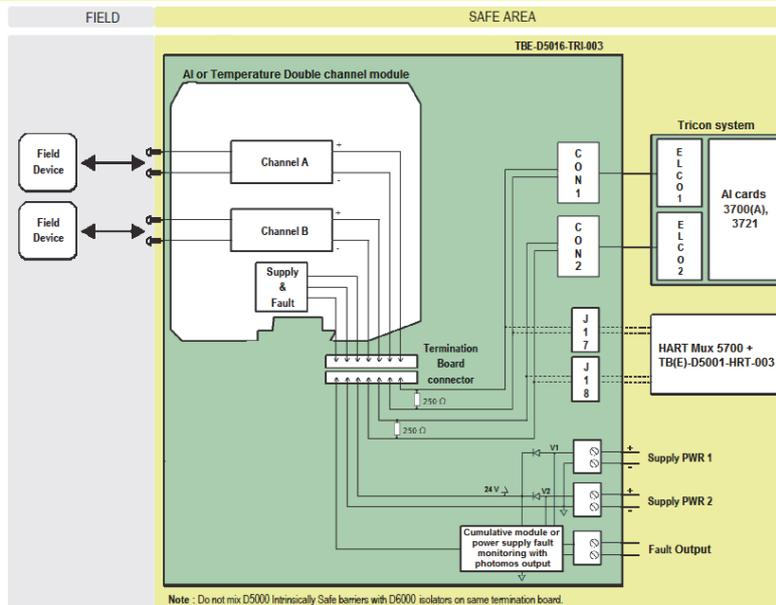
The diagram shows a double channel module on TBE. On a single TBE-D5016-TRI-003 Termination Board can be installed up to 16 double ch. modules for a maximum of 32 channels.
