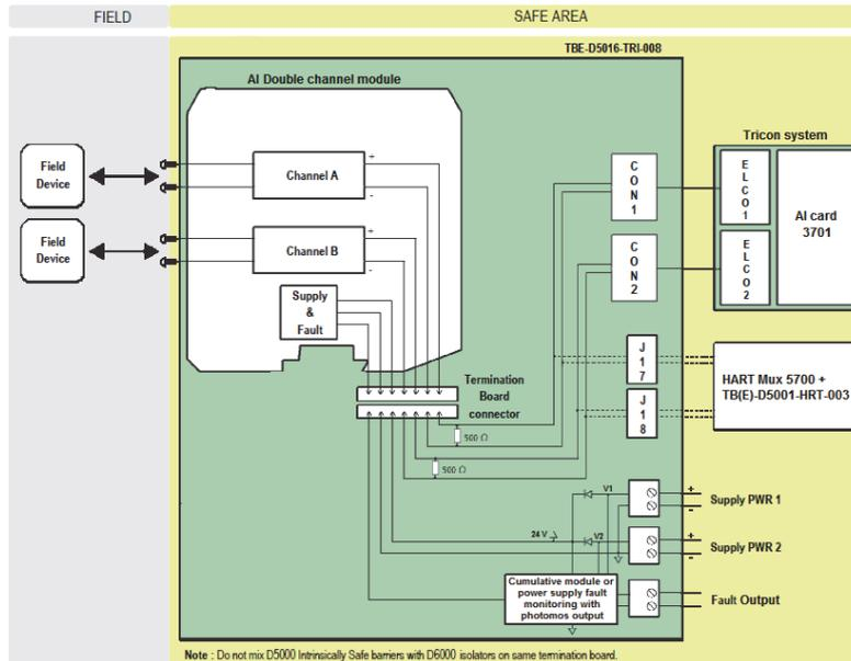
The diagram shows a double channel module on TBE. On a single TBE-D5016-TRI-008 Termination Board can be installed up to 16 double ch. modules for a maximum of 32 channels.
