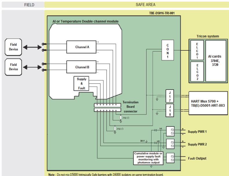
The diagram shows a double channel module on TBE. On a single TBE-D5016-TRI-001 Termination Board can be installed up to 16 double ch. modules for a maximum of 32 channels.
