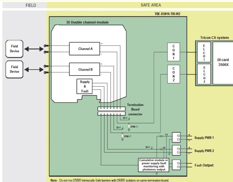
Note : Do not mix D5000 Intrinsically Safe barriers with D6000 isolators on same termination board.
