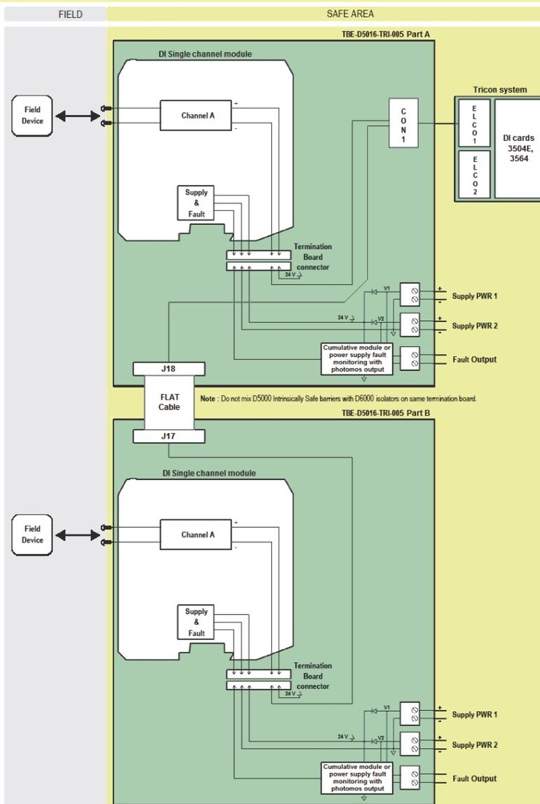
The diagram shows a single channel module on each TBE Part A or Part B.
