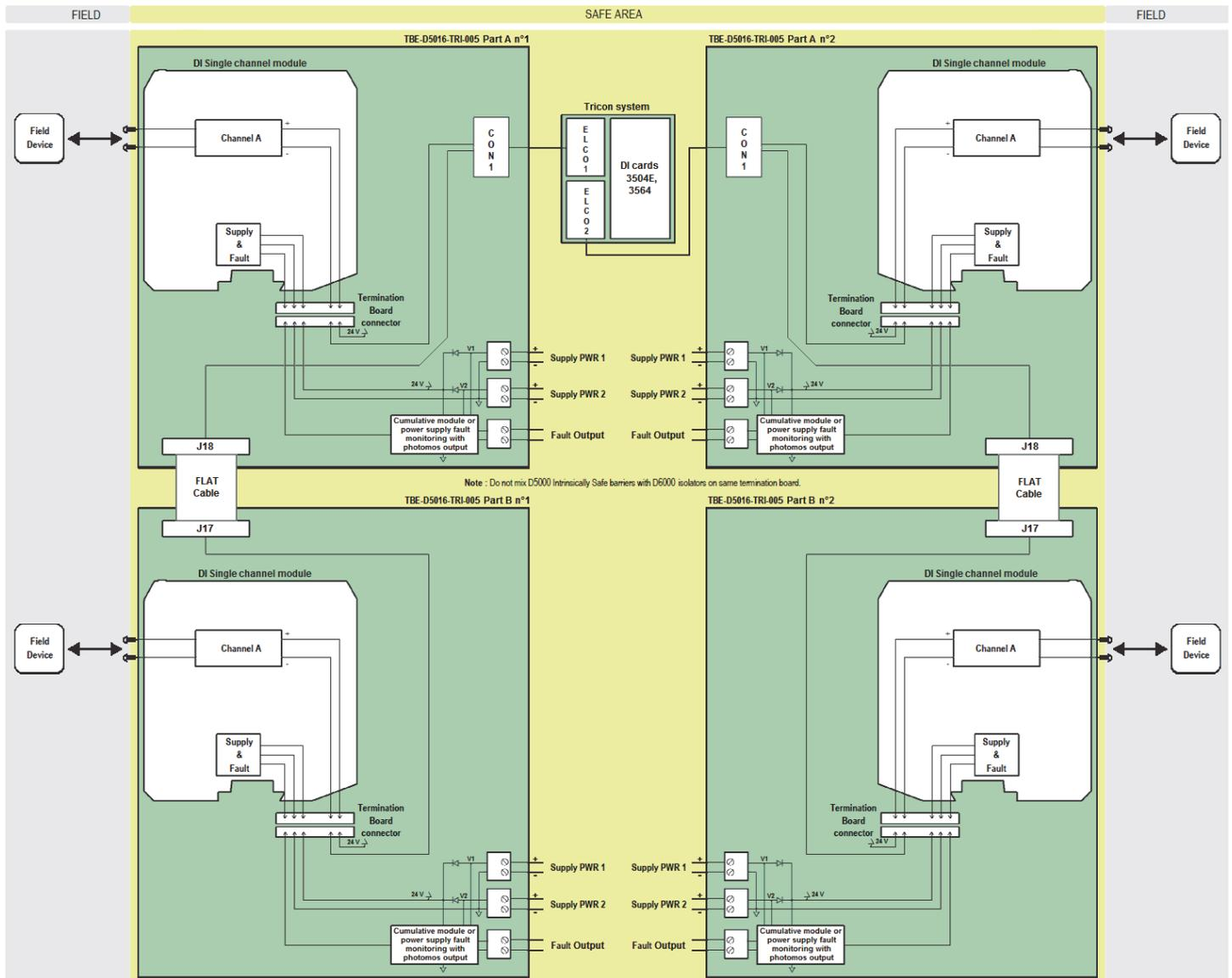
The diagram shows a single channel module on each TBE Part A or Part B.
