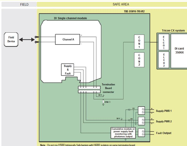
The diagram shows a single channel module on TBE. On a single TBE-D5016-TRI-012 Termination Board can be installed up to 16 single ch. modules for a maximum of 16 channels.
