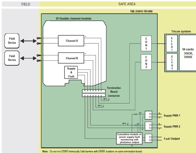
The diagram shows a double channel module on TBE. On a single TBE-D5016-TRI-006 Termination Board can be installed up to 16 double ch. modules for a maximum of 32 channels.
