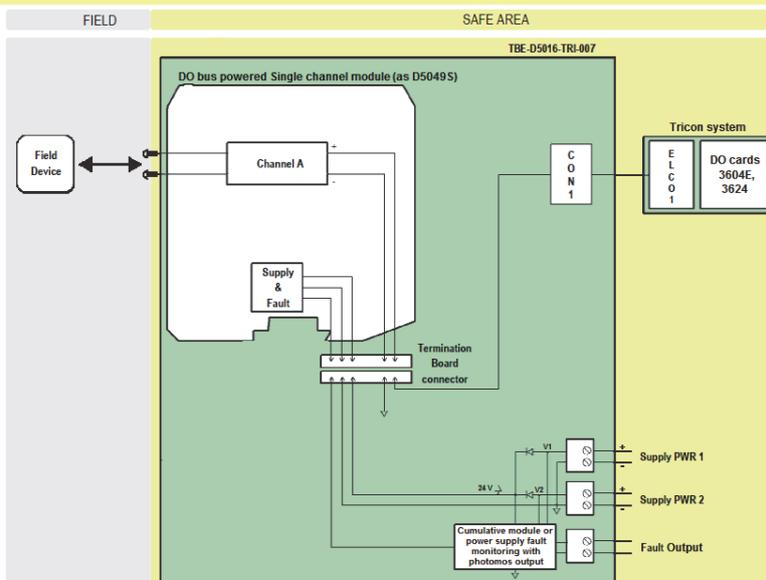
The diagram shows a single channel module on TBE.
