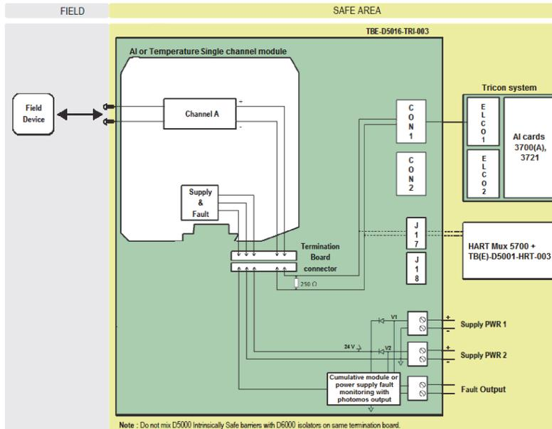
The diagram shows a single channel module on TBE. On a single TBE-D5016-TRI-003 Termination Board can be installed up to 16 single ch. modules for a maximum of 16 channels.
