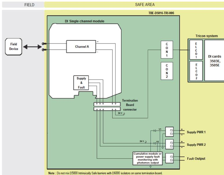
The diagram shows a single channel module on TBE. On a single TBE-D5016-TRI-006 Termination Board can be installed up to 16 single ch. modules for a maximum of 16 channels.
