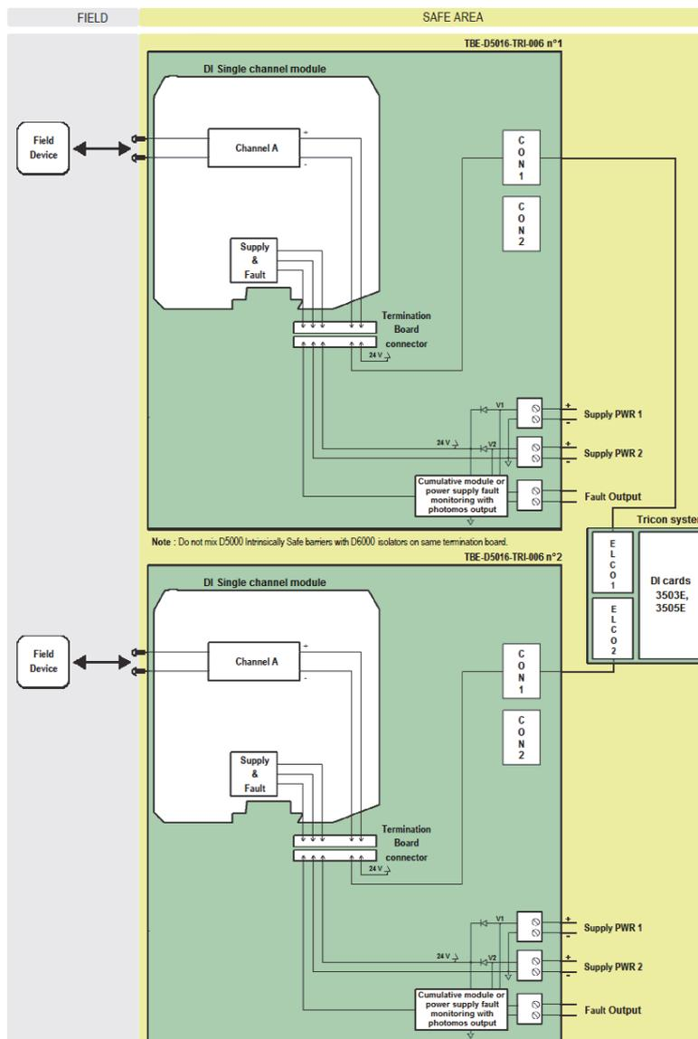
The diagram shows a single channel module on each TBE. On two TBE-D5016-TRI-006 Termination Boards can be installed up to 16+16 single channel modules for a maximum of 32 channels.
