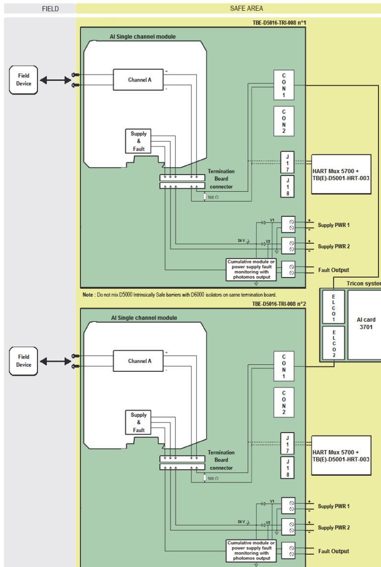
The diagram shows a single channel module on each TBE. On two TBE-D5016-TRI-008 Termination Boards can be installed up to 16+16 single channel modules for a maximum of 32 channels.
