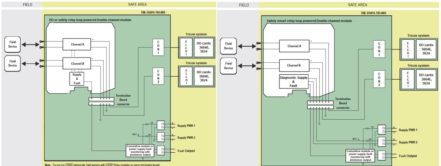
Each diagram shows a double channel module on TBE.
