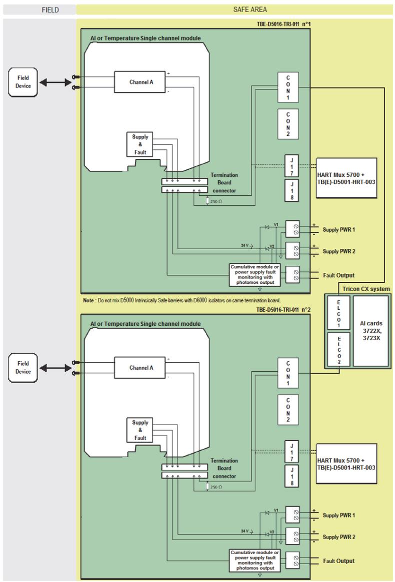
The diagram shows a single channel module on each TBE. On two TBE-D5016-TRI-011 Termination Boards can be installed up to 16+16 single channel modules for a maximum of 32 channels.
