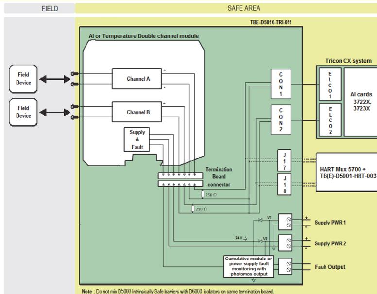
The diagram shows a double channel module on TBE. On a single TBE-D5016-TRI-011 Termination Board can be installed up to 16 double ch. modules for a maximum of 32 channels.
