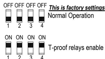
**WARNING:** after T-proof test, dip-switch 1-2-3-4 **must be set** to "OFF" position for normal operation.
