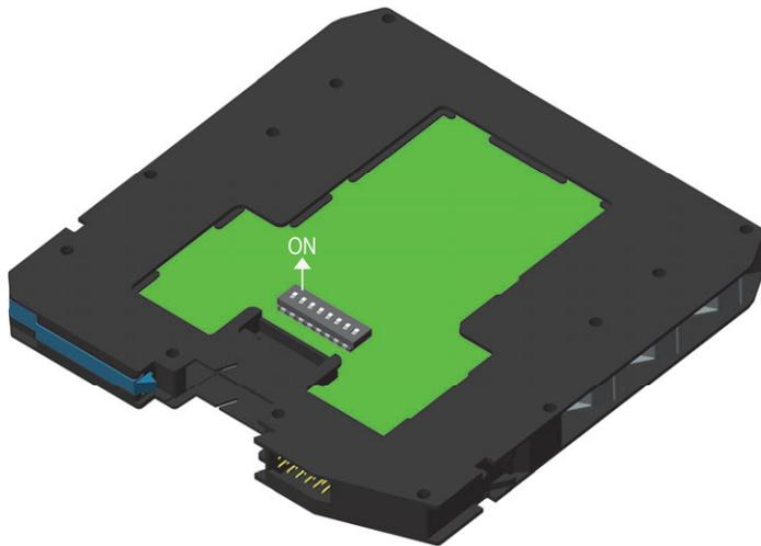
Dip switch factory settings. All Switches are OFF
