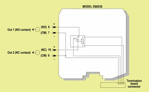
Relay contacts shown in de-energized position. Terminals 7-8 are open; terminals 9-10 are closed.
