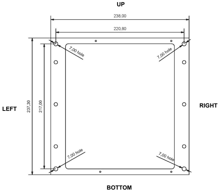
The following drawing with overall dimensions (mm) is only applicable to types: PSS1250-HS-2 and PSS1250-2.
