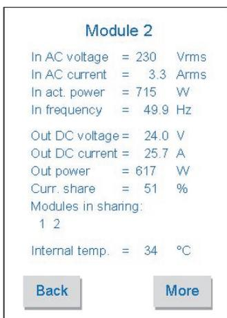
Touching "2 POS" cell on the main menu screen, PSM1250 module 2 (Pos.2) first page data are shown. Modules 1 and 2 are in sharing. Touch "Back" cell to return on the main menu or touch "More" cell to go on the module second page data.
