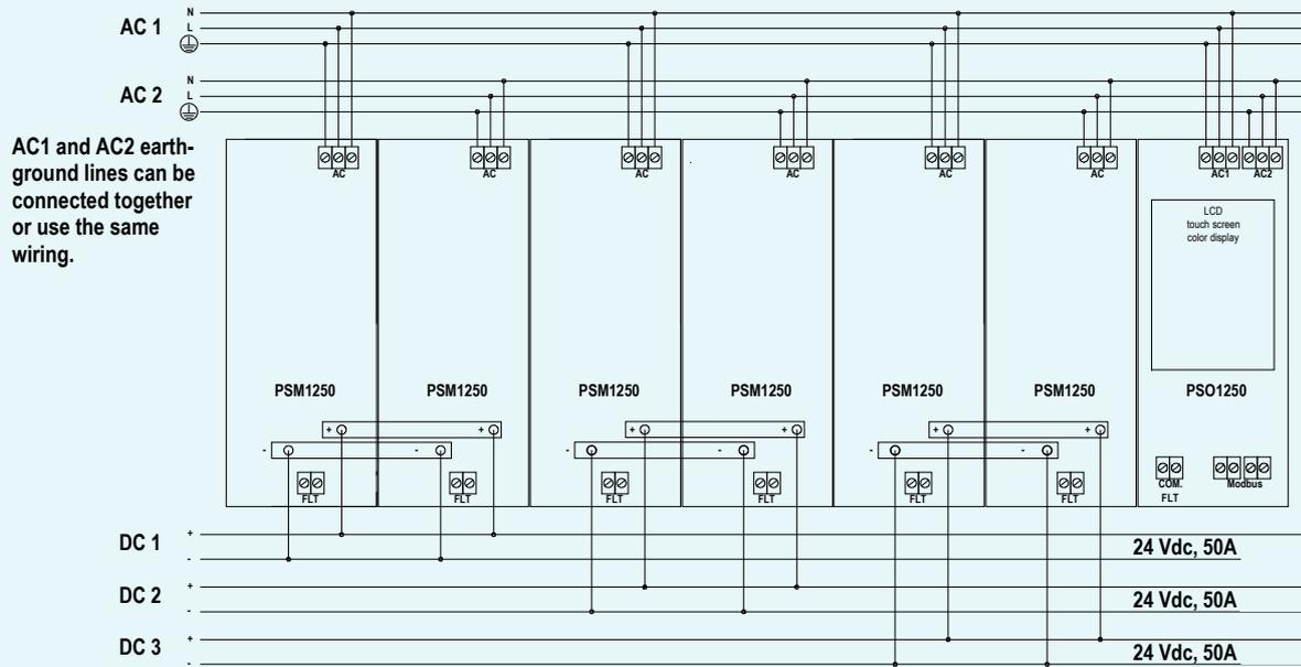
If electrical isolation between paralleled output groups is not required, DC 1 (-), DC 2 (-) and DC 3 (-) negative lines can be connected together or use the same wiring.
