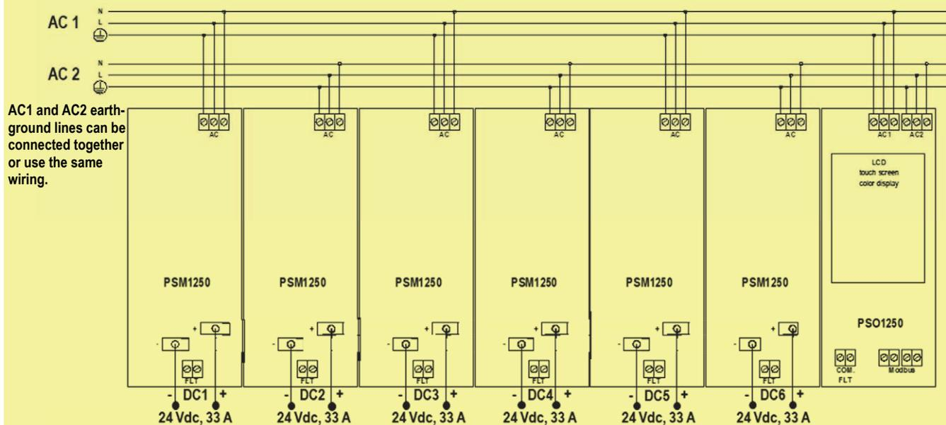
Back Panel PCB of PSS1250-HS-7-0-D or PSS1250-HS-7-5-D with Hot Swapping circuits:
