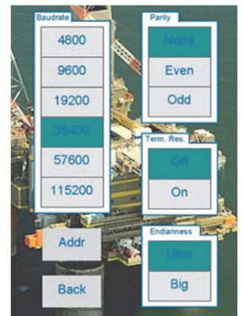
This image is shown when touching the "Modbus" cell in the set up menu screen. Here is possible to set Modbus communication parameters as baudrate, parity, terminal resistance, endianness and address, touching related cells. These parameters are saved in PSO1250 memory and also held after AC1 and AC2 supply shutdown.
