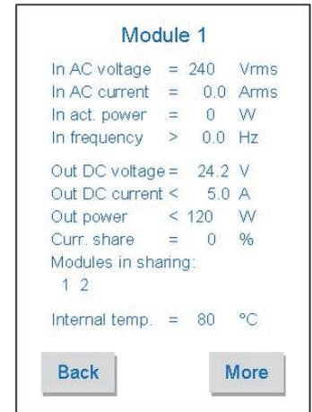
Indeed, module 1 internal temperature is 80°C, higher than 75°C. The module has thermal hysteresis and it removes internal temperature over-range fault when its internal temperature is reduce under 70°C. AC line is present and its voltage is 240 Vrms. Module 1 does not contribute to supply the 1 & 2 group load and its out current sharing percentage is 0%.
