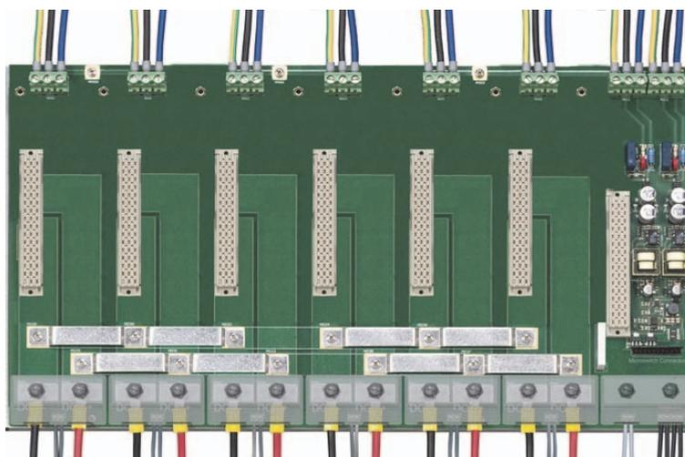
**Function Diagram Dual AC Supply wiring architecture for PSS1250-HS-3-D or PSS1250-3-D fully equipped:**
