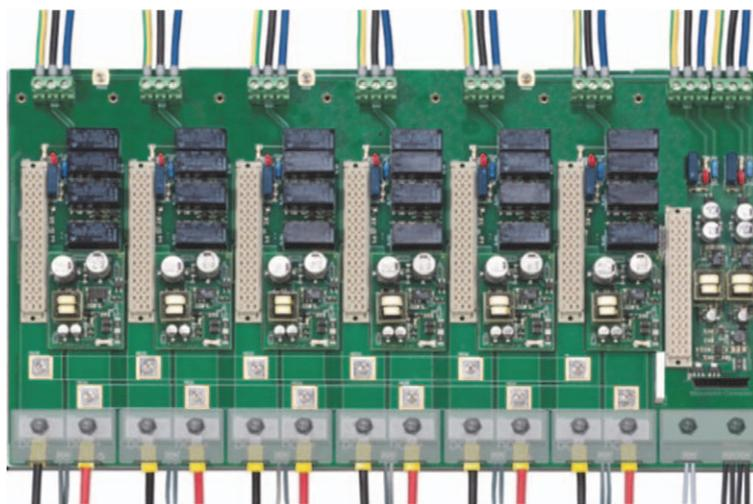
Back Panel PCB of PSS1250-7-0-D or PSS1250-7-5-D without Hot Swapping circuits:
