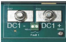
For all configurations except PSS1250(-HS)-7-0 & -7-5 PSM1250 screw output terminals on copper bars: DC- is negative out pole, DC+ is positive out pole. (in the figure it's shown DC1- and DC1+ which are related to PSM1250 in position 1 of PSS1250 system).
