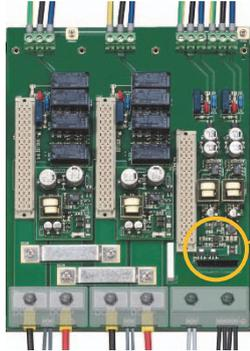
During installation of the PSS1250-HS-7-x-D or PSS1250-HS-3-D, connect the flat cable, coming from the microswitches PCB of the Rack unit, to the 12 poles male connector on Back Panel PCB, as shown in Fig. 6-7.
