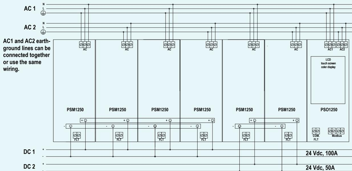
If electrical isolation between paralleled output groups is not required, DC 1 (-) and DC 2 (-) negative lines can be connected together or use the same wiring.
