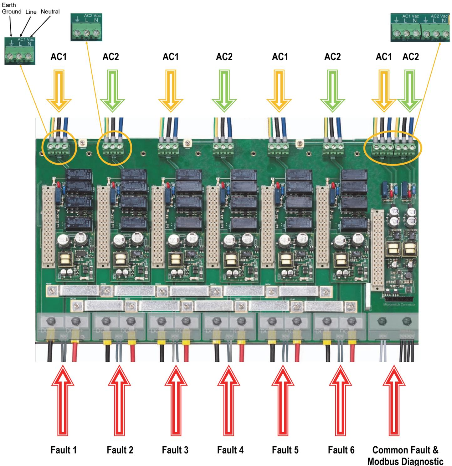
The PSS1250 redundant system requires to use two AC input power lines (AC1 and AC2) with different lines and neutrals but the same Earth Ground connection, in order to guarantee fully redundant configuration from the input to the output of power system. For PSS1250(-HS)-7-0 & -7-5 not redundant system, it is not required two AC input power lines. Each PSM1250 unit slot must receive AC mains by means of a circuit breaker or switch with the following features:
