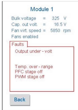
The PSM1250 module 1 (Pos.1) is in fault condition because of: internal temperature over-range, which imposes thermal shutdown of internal PFC and PWM stages, implying output under-voltage (16.5 V < 20 V bottom limit). Note that AC line is present and fans go on to work at low speed in order to cool whole module.
