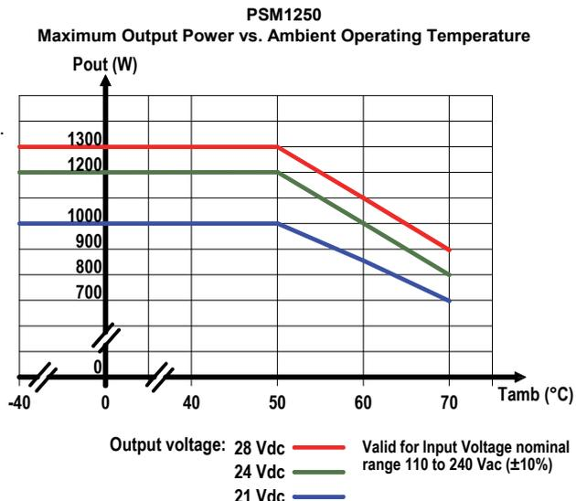
With 50% redundant configuration (two PSM1250 with paralleled outputs), each module can give 600 W power output up to 70°C operating ambient temperature, with output voltage range 21÷28 Vdc and input voltage nominal range 110÷240 Vac ( $\pm 10\%$ ).
