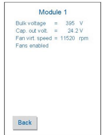
This is PSM1250 module 1 (Pos.1) second page where other data are shown: Bulk Voltage or internal PFC capacitor voltage, Capacitor out voltage or out voltage before active ideal diode, Fan virtual (or set) speed, indication if fans are enabled or disable. In addition, this page is used to show fault alarm as: under/over out voltage, AC line absence, internal PFC or PWM stage in OFF state, internal high temperature, fans malfunction). Touch "Back" cell to return on the module first page.
