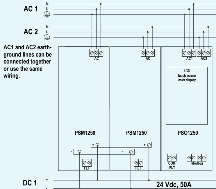
**Back Panel PCB of PSS1250-HS-3-D with Hot Swapping circuits:**
