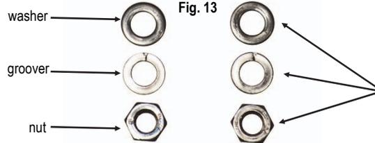
Unplug M6 nuts, groovers and washers. Then insert a cable lug (at least 6.5 mm hole diameter) with wire, washer and groover on each screw output terminal. Finally tighten nut to fix wire.
