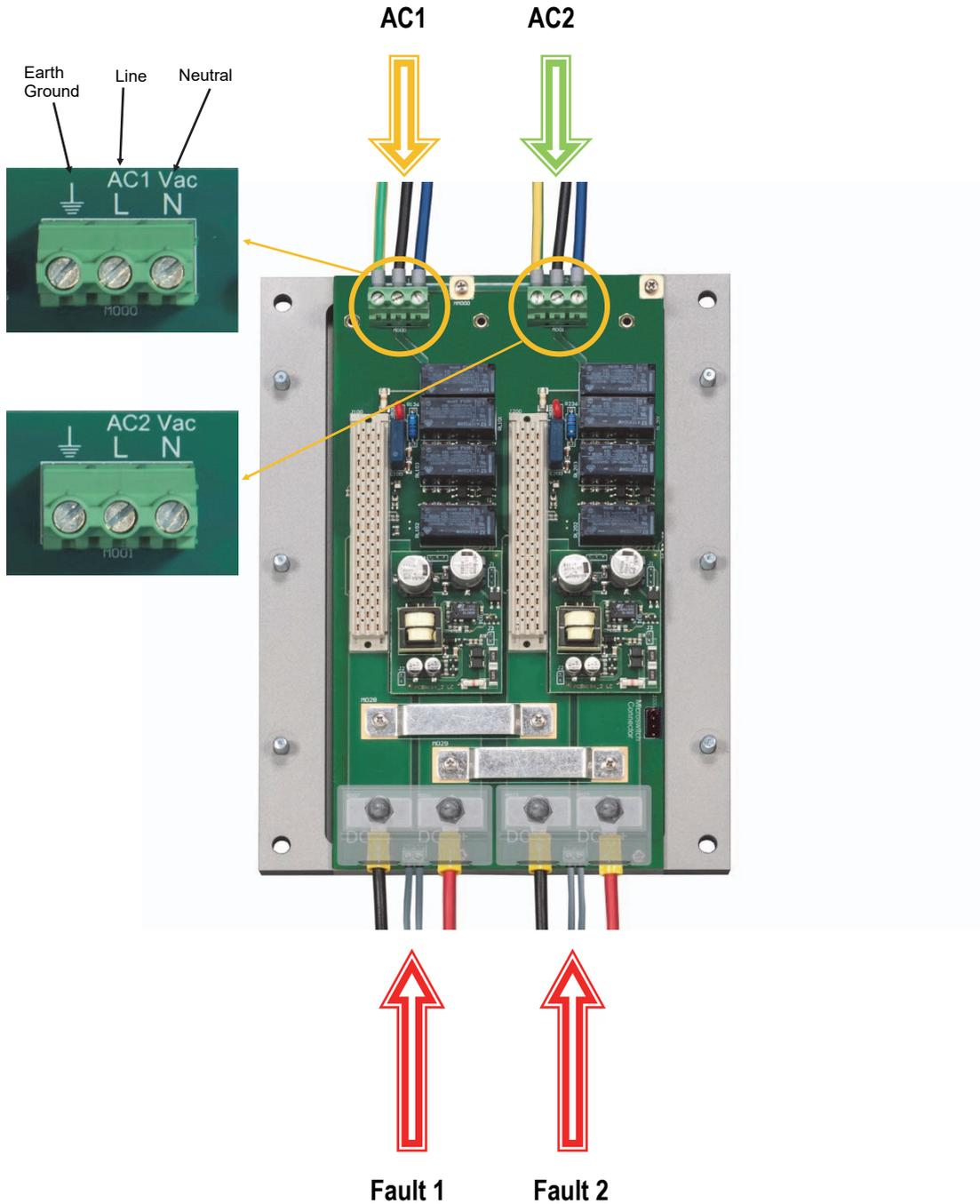
The PSS1250 redundant system requires to use two AC input power lines (AC1 and AC2) with different lines and neutrals but the same Earth Ground connection, in order to guarantee fully redundant configuration from the input to the output of power system.
