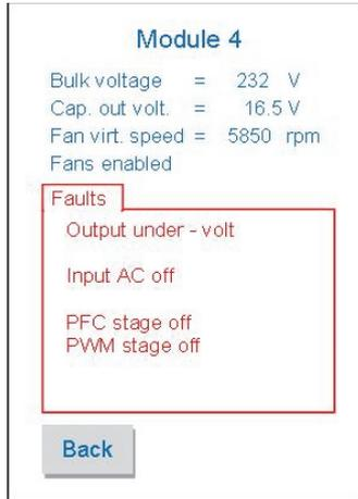
The PSM1250 module 4 (Pos.4) is in fault condition because of: AC line absence which implies internal PFC and PWM stages in OFF state and output under-voltage (16.5 V < 20 V bottom limit).
