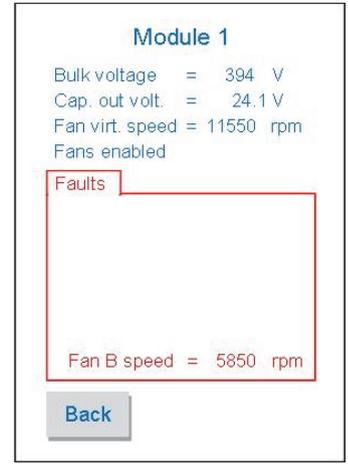
The fault is due to Fan B malfunction, because its speed is 5850 < 11550 rpm setting, that is Fan B works but not correctly. When speed difference between setting speed value and read speed value is more in absolute to 5000 rpm a fan fault is shown, specifying speed reading.
