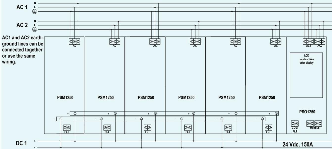
**Back Panel PCB of PSS1250-HS-7-1-D or PSS1250-HS-7-6-D with Hot Swapping circuits:**
