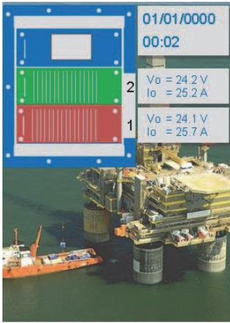
The PSM1250 module 1 (Pos.1) is in fault condition because its "1 POS" cell on the main menu screen is red. Its Vo out voltage before active ideal diode and its Io out current are seemingly correct. The answer is shown in the module second page, which resumes fault alarms.
