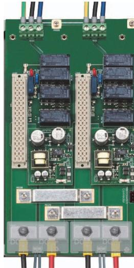
**Back Panel PCB of PSS1250-2 without Hot Swapping circuits:**
