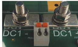
Only for PSS1250(-HS)-7-0 & -7-5 PSM1250 screw output terminals on copper bars:
