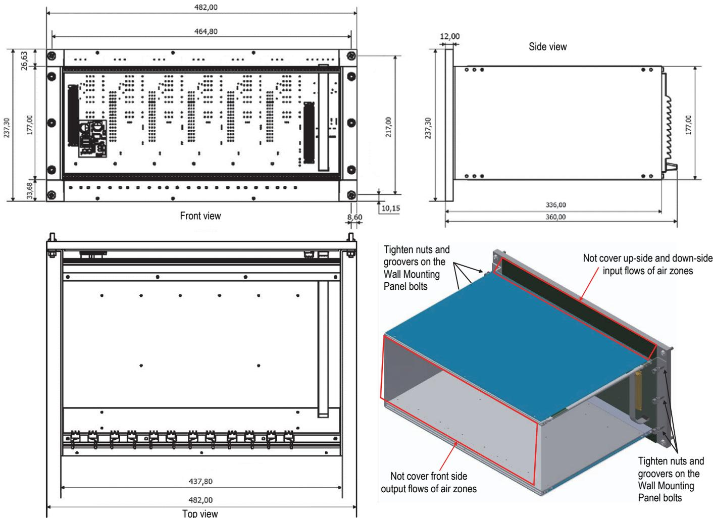
**Installation Procedure - 3rd step: Rack unit installation on Back Plane for PSS1250-xx-3-D (for wall mounting into a cabinet)**
