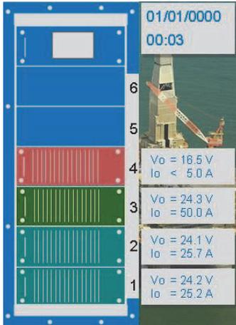
The PSM1250 module 4 (Pos.4) is in fault condition because its "4 POS" cell on the main menu screen is red. Its Vo out voltage before active ideal diode is 16.5 V < 24.3 V and its Io out current is < 5 A < 25.5 A . Therefore module 4 does not contribute to supply the 3 & 4 group load. Now, only module 3 (Pos.3) drives the 3 & 4 group load because its Io out current is increased from 25.4 to 50.0 A.
