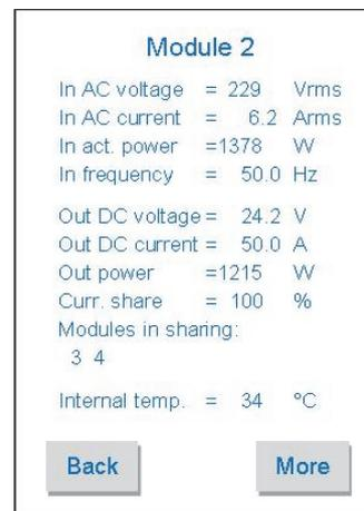
The PSM1250 module 2 (Pos.2) drives the 1 & 2 group load because its Io out current is increased from 25.7 to 50.0 A and its out current sharing percentage is 100%.
