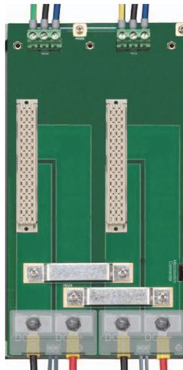
1) Application of PSS1250 with HS and single PSM1250 module, for NE output load
