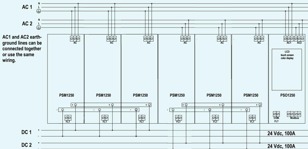
If electrical isolation between paralleled output groups is not required, DC 1 (-) and DC 2 (-) negative lines can be connected together or use the same wiring.
