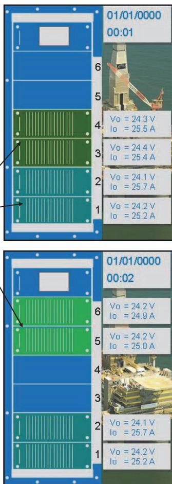
All PSM1250 modules are normally operating (their pos. cells are all green). This image is related to PSS1250-xx-7-3-D because there are 3 current sharing groups: 1 & 2 ; 3 & 4 ; 5 & 6 . For each operating PSM1250 module, on the right of its "x POS" cell, there is a label that shown: - Vo , its out voltage before active ideal diode (which is different from out DC or out group voltage); - Io , its out current or out DC current.
