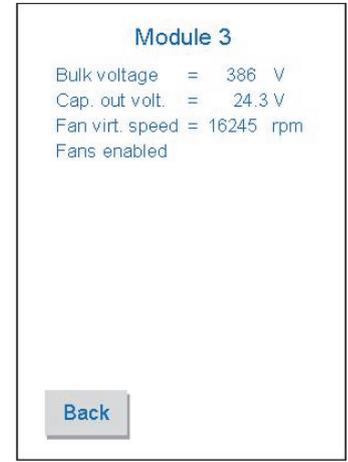
Now, Fan virtual (or set) speed is increased from 11540 to 16245 rpm because of out power increment. Indeed, fan speed control depending on output power and ambient temperature.
