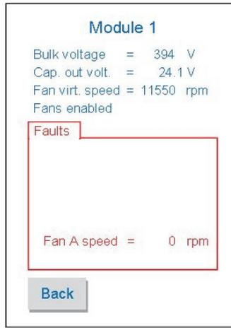
The fault is due to Fan A malfunction, because its speed is 0 < 11550 rpm setting, that is Fan A does not work.
