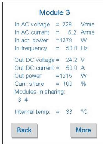
The PSM1250 module 3 (Pos.3) drives the 3 & 4 group load because its Io out current is increased from 25.4 to 50.0 A and its out current sharing percentage is 100%.
