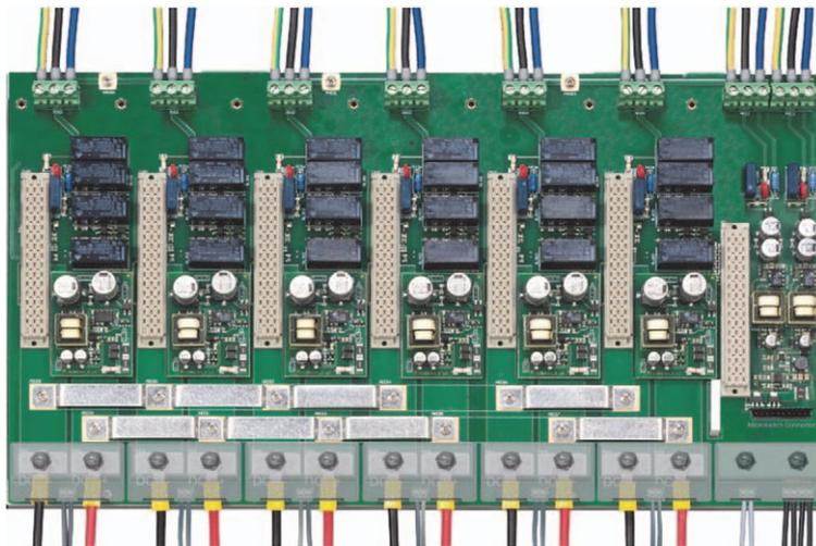
**Back Panel PCB of PSS1250-7-2-D or PSS1250-7-7-D without Hot Swapping circuits:**
