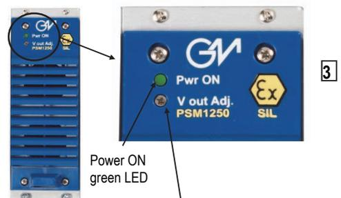
The new PSM1250 module is powered and its green LED is ON, but the module is not operating in current sharing with other PSM1250 modules paralleled with it, because its output voltage is too low (21 Vdc).
