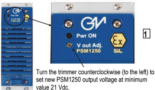
Then insert and fix the new PSM1250 module into the Rack unit by means of its 4 screws on front side. First tighten 2 bottom screws and then tighten 2 top ones.
