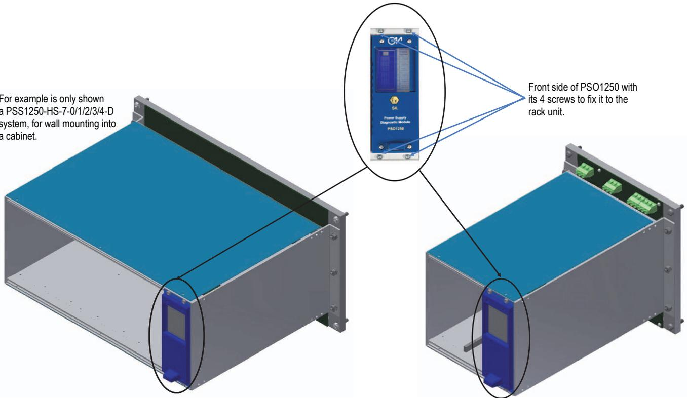
Front side of PSO1250 with its 4 screws to fix it to the rack unit.
