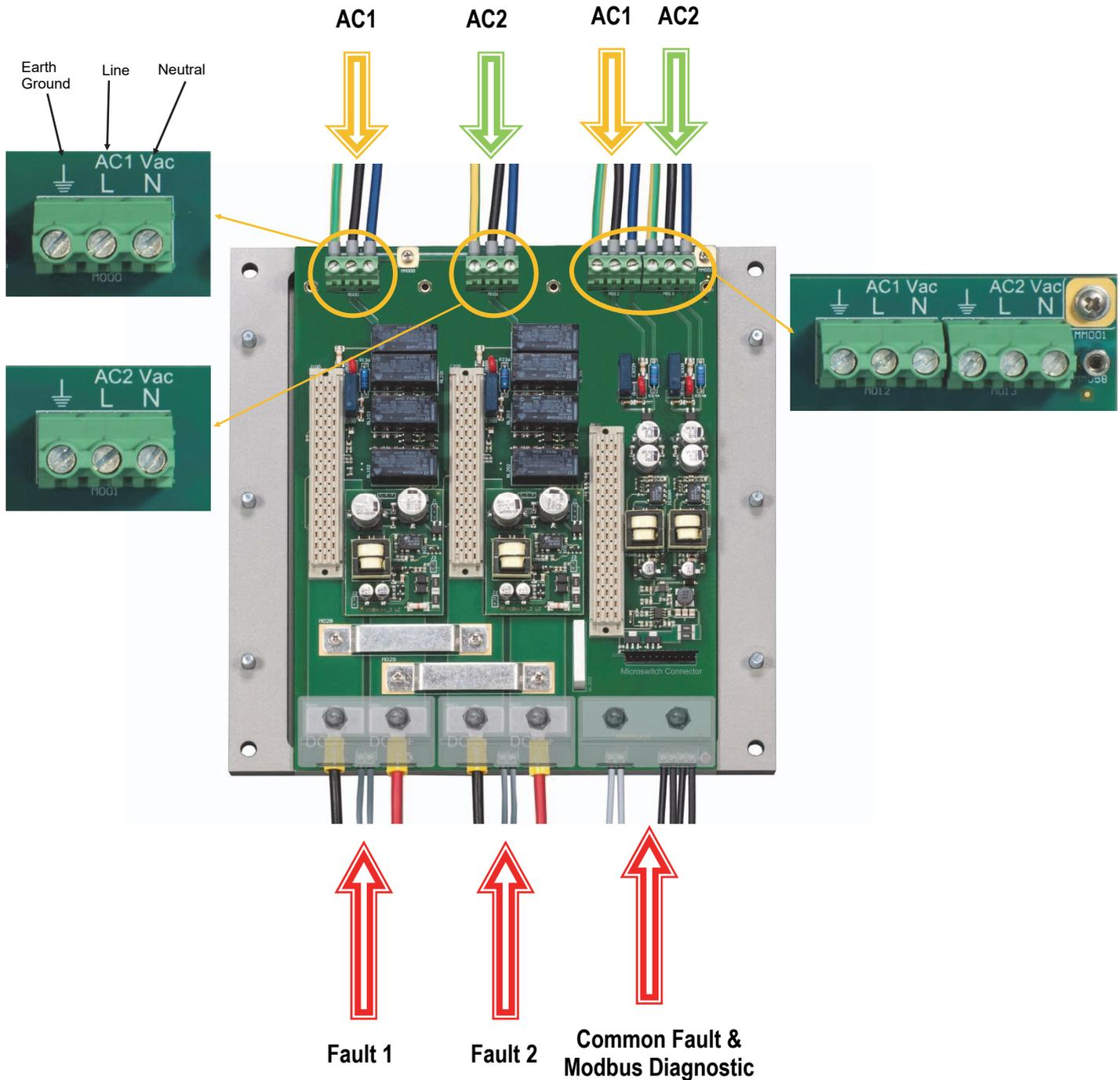
The PSS1250 redundant system requires to use two AC input power lines (AC1 and AC2) with different lines and neutrals but the same Earth Ground connection, in order to guarantee fully redundant configuration from the input to the output of power system.
