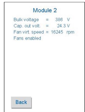
Now, Fan virtual (or set) speed is increased from 11550 to 16245 rpm because of out power increment. Indeed, fan speed control depending on output power and ambient temperature.
