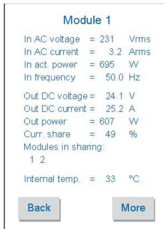
Touching "1 POS" cell on the main menu screen, PSM1250 module 1 (Pos.1) first page data are shown: Input AC Voltage and Current, Input Active Power, Input Line Frequency, Output DC or out group Voltage (after active ideal diode), Output DC Current, Output Power, Output current sharing percentage, Current sharing group (modules 1 and 2 are in sharing), Internal Temperature. Touch "Back" cell to return on the main menu or touch "More" cell to go on the module second page data.
