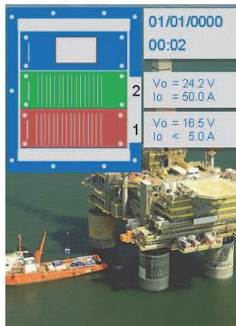
The PSM1250 module 1 (Pos.1) is in fault condition because its "1 POS" cell on the main menu screen is red. Its Vo out voltage before active ideal diode is 16.5 V < 24.3 V and its Io out current is < 5 A < 25.2 A. Therefore module 1 does not contribute to supply the 1 & 2 group load. Now, only module 2 (Pos.2) drives the 1 & 2 group load because its Io out current is increased from 25.7 to 50.0 A.
