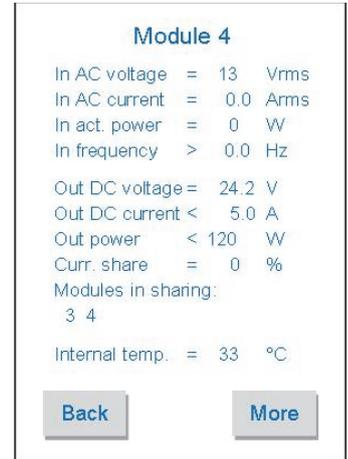
Capacitor out voltage or out voltage before active ideal diode is 16.5 V but out DC or out group voltage (after active ideal diode) is 24.2 V. Module 4 does not contribute to supply the 3 & 4 group load and its out current sharing percentage is 0%. Out current and power measure at low load (< 5 A) is not accurate so that: Out DC current < 5 A and Out power < 120W.
