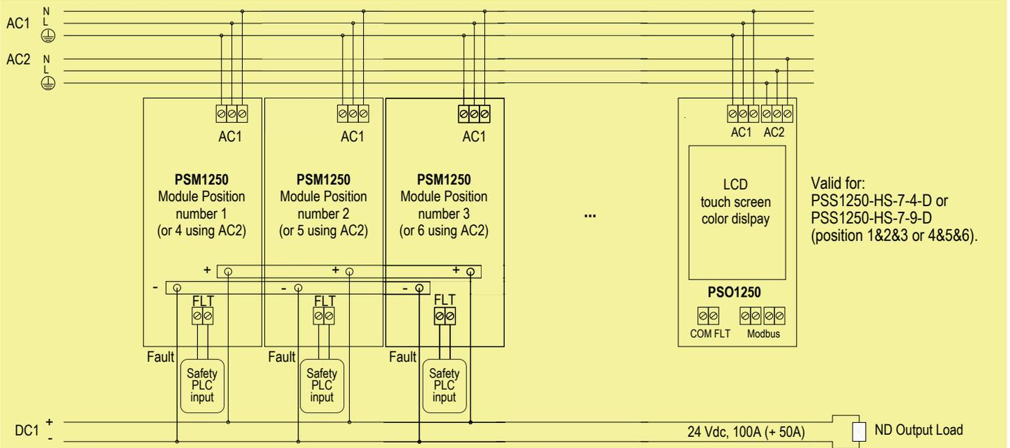
**Description:** In normal operation three paralleled PSM1250 modules (1st, 2nd and 3rd ones) are unpowered because of absence of only AC1 input supply (for 4th, 5th and 6th modules use AC2 input supply line), which is connected by means of related terminal blocks on the Back Panel PCB (see previous functional diagram for more information).
