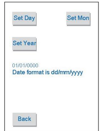
This image is shown when touching the "Set Date" cell in the set up menu screen. Here is possible to set Day, Month and Year touching related cells. Date format is day/month/year (as dd/mm/yyyy). Current setting is shown in numeric format. Date is not kept after AC1 and AC2 supply shutdown.
