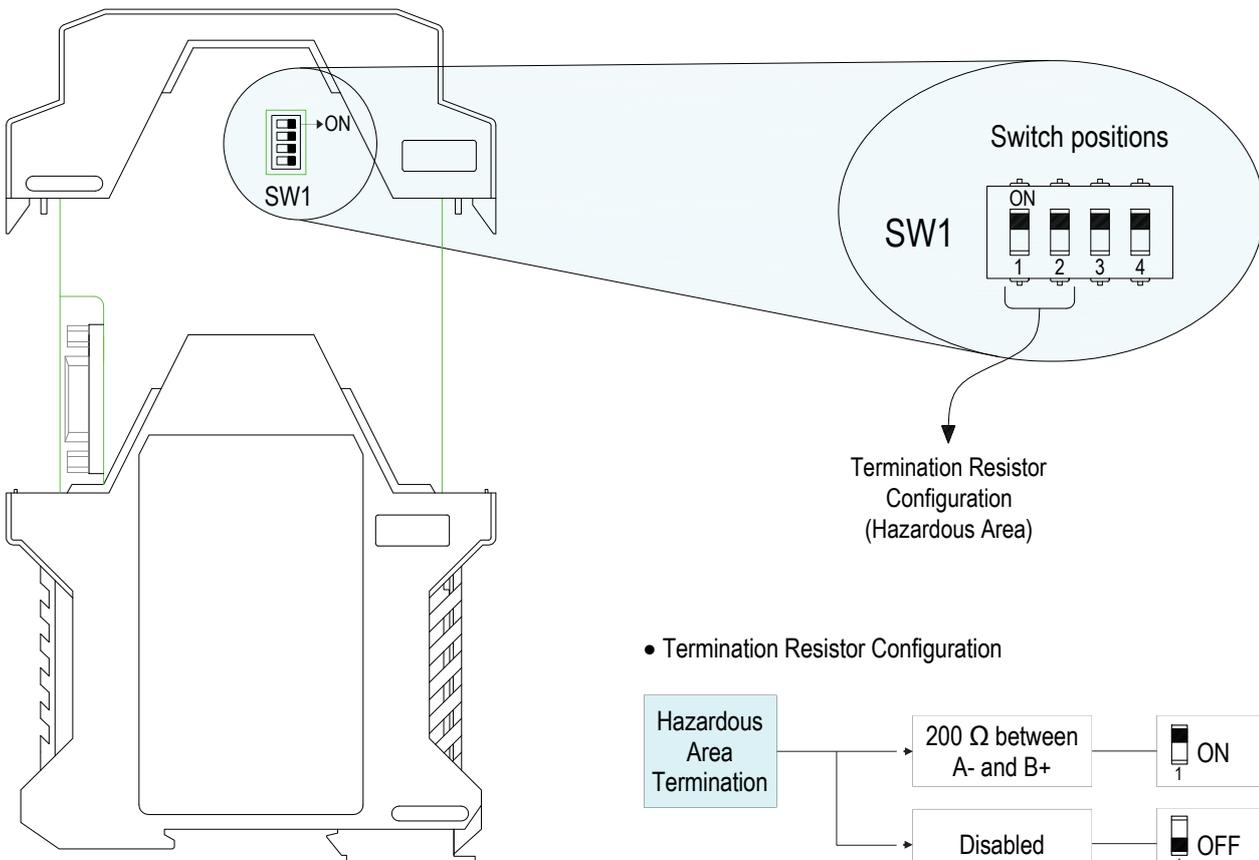
• Termination Resistor Configuration
