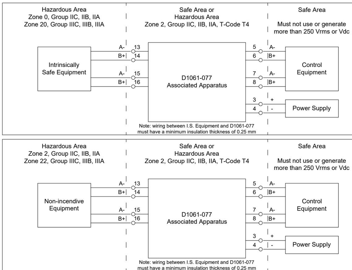
The wiring between the Intrinsically Safe Equipment located in Hazardous Area and the D1061-077 Associated Apparatus must have a minimum insulation thickness of 0.25 mm. Not to be connected to control equipment that uses or generates more than 250 Vrms or Vdc with respect to earth ground.
