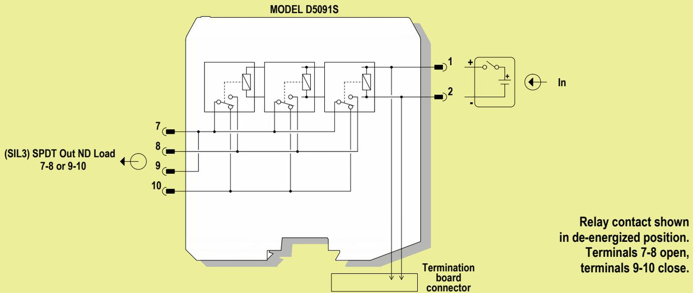
**SIL3 Safety Function for ND load (energized in fail safe state) is available at terminal blocks 7-8;
