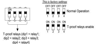
WARNING: after T-proof test, dip-switch 1-2-3-4 must be set to "OFF" position for normal operation.
