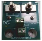
PSW1250 screw output terminals on copper bars: DC- is negative out pole, DC+ is positive out pole.
