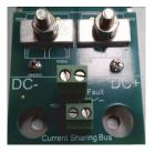
disconnect cable lug with wire from each screw output terminal.
