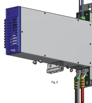
After wiring of the DC output lines and current sharing bus, **power AC1 and AC2 input power lines**. Therefore, each PSW1250 turns on and the whole power system can drive the loads connected to the DC output lines.
