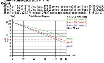
Short circuit current: ≥ 50 mA (55 mA typical). Response time: ≤ 10 ms
